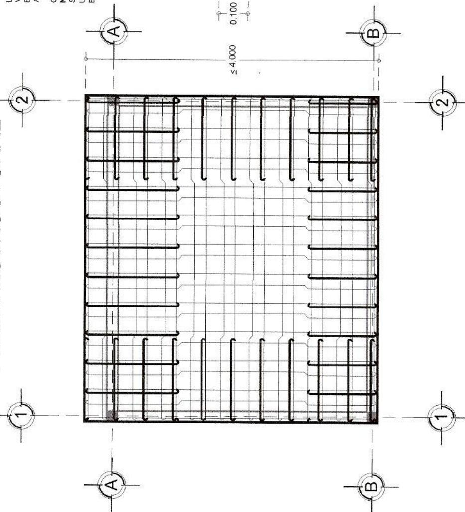
LOSA CONCRETO FC 200KG/CM<sup>2</sup> 10 CMS ESPESOR
